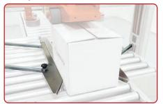
**GUIDE RAIL MECHANISM** Positions the carton within the machine to ensure an even seal on both the top and bottom of the carton. via a QR code on solution.
