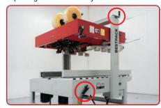
Manually adjust the top mast and side belts based to get the right fit for your carton.
