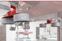
**TOP COMPRESSION ROLLERS** Eliminates the carton's top gap for added product security.
