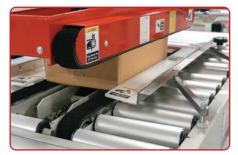
**2 TOP & 2 BOTTOM BELT DRIVES** Top and bottom belts ensure a stable throughput for cartons, ensuring a clean seal.
