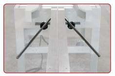
**BOTTOM FLAP FOLDER** Eliminates repetitive manual folding of bottomflaps, improving worker efficiency.
