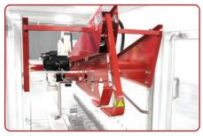
**TOP FLAP FOLDING KICKER & HORNS** Eliminates manual folding of top flaps, boosting throughput and efficiency.
