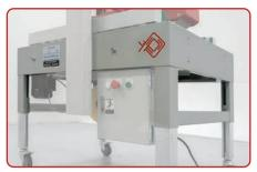
**CNC CUT AND WELDED FRAME/LEGS**
