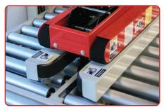
**2 TOP AND 2 SIDE BELT DRIVES** Gently pulls product through while reducing less wear & tear on parts.
