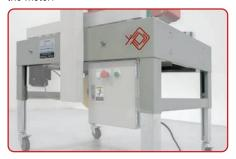
**CNC CUT AND WELDED FRAME/LEGS**
