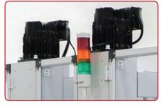
**DUAL SERVO MOTORS POWERED** Provides precise control of position and speed on the Flap Folding Station and Sealing Station.
